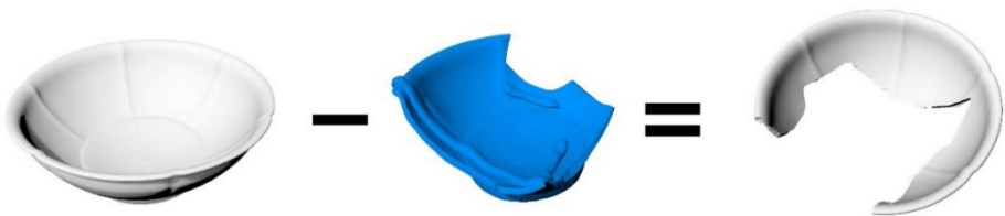
Fig. 5 Schematic illustration of the Boolean operation
