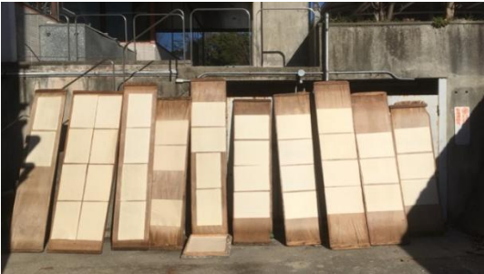
Fig. 10 Itaboshi of Kozo paper (method of drying Kozo paper by pasting it onto wooden boards and exposing it to sunlight).
