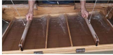
Fig. 14 Sheet formation (Papermaking) process using the Neri effect (left and right).
