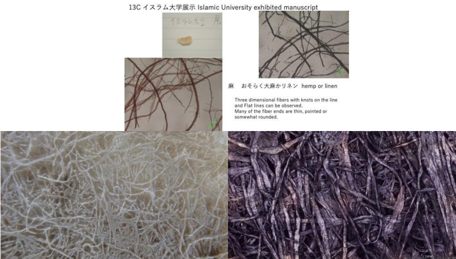
Fig. 34 Paper fragment from an Islamic manuscript (Linen/Hemp paper), Graff C stain (top), image from a simple still camera (left), and image from a white light confocal microscope (right).
