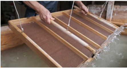
Fig. 14 Sheet formation (Papermaking) process using the Neri effect (left and right).
