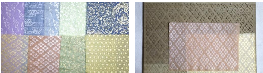
Fig. 18 Samples of dyeing and Kirazuri (mica printing) (left), and woodblocks used for Karakami (printed paper) (right).
